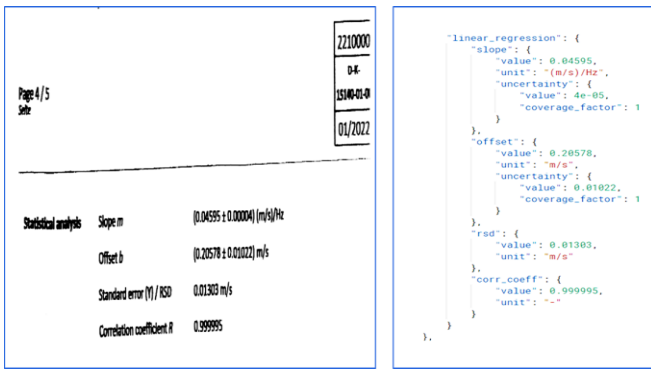
Figure 2. Example of analogue calibration certificate and its DCC counterpart excerpt. Figure shows that the mistakes that might happen in the analogue certificate, e.g. due to OCR, is not possibly happen in the DCC.
