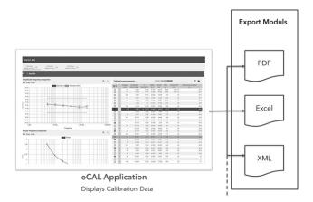
Fig. 3: A new application works as a middleware that allows to display the calibration results and transform it via export modules into several output formats
