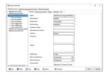
Fig. 2: The DUT database allows to manage an unlimited number of measurement channels / axis for each DUT. Each channel / axis can measure a different measurand.
