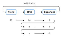
Fig. 2 Example for an algorithmic representation of units of measurement, which can be used by a software
