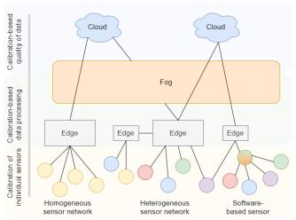
Fig. 1 Calibration information in the different layers of the IoT architecture.
